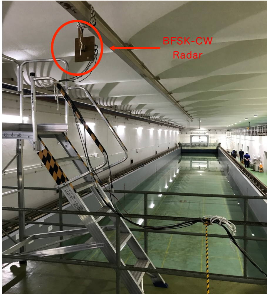
Fig.14 Experimental landscape of ship model basin and BFSK-CW Radar.
