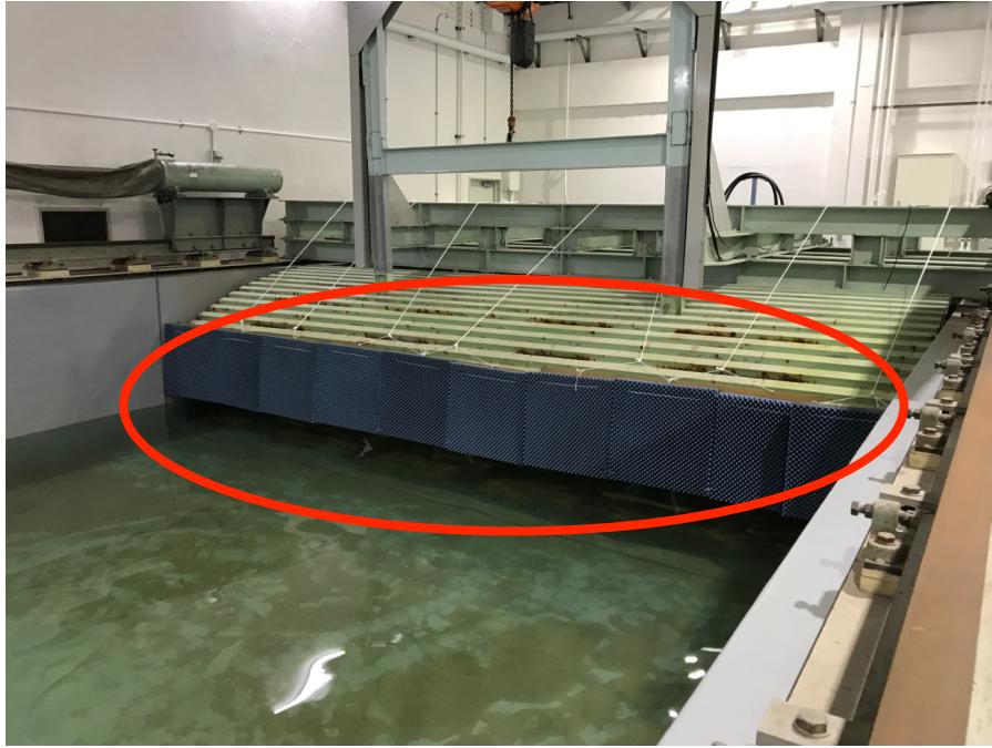
Fig.15 Electromagnetic wave absorption material in front of wave-making equipment.
