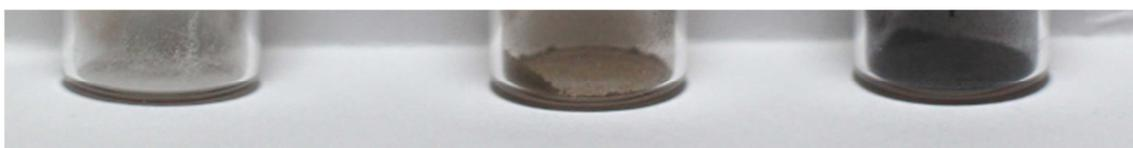
Fig.16 Photographs of cellulose powder heated by TG up to 200°C (left), 300°C (center), 400°C (right)
